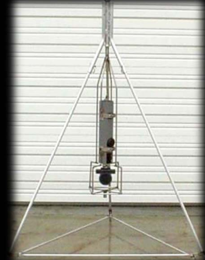
Tripod mounting for stationary, free standing deployment
